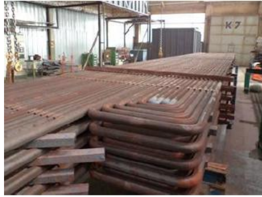
Recovery boiler: Super heater (Finland)
